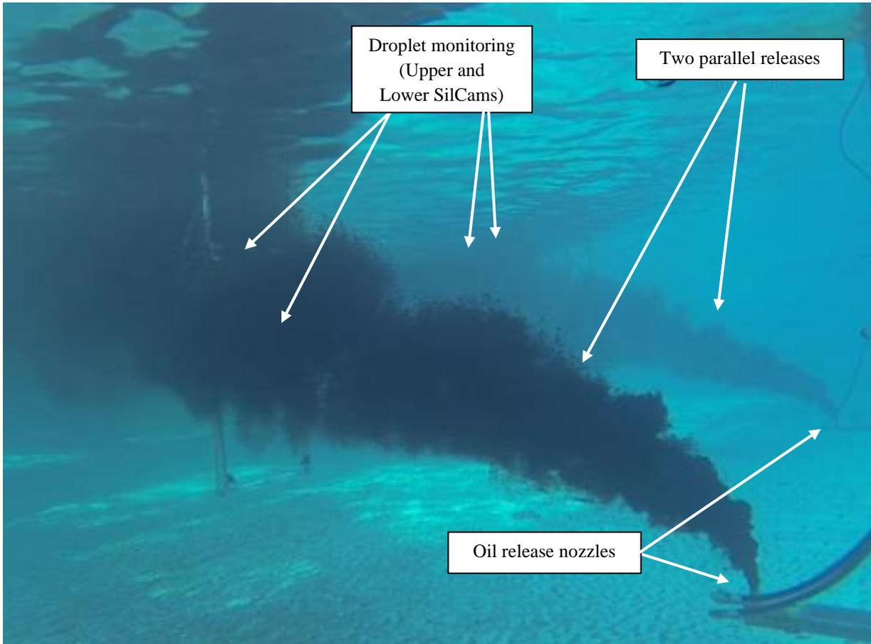
Figure 1: Twin releases of oil from the two different nozzle configurations illustrate plume behaviour and position of monitoring equipment. Two set of SilCams were used to monitor oil droplet sizes in both oil plumes. The closest release arrangement could switch between two different release nozzles (32 mm or 50 mm), the other had a fixed nozzle size (25 mm). From Brandvik et al., 2021.
