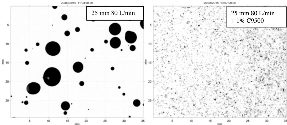
Figure 2: SilCam images showing individual droplets (25 mm nozzle, 80 L/min and 80 L/min with 1% C9500. From Brandvik et al., 2021.
