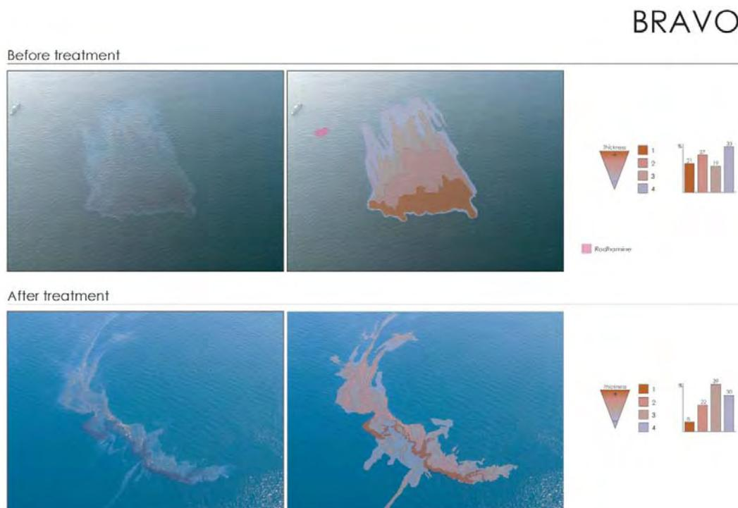
Slick C was treated by the ship Lynx for 1 hour and 10 minutes. The dispersant was applied neat with an adjustable flow rate spraying equipment of the French Navy; this equipment is composed of 3 spraying assemblies, which can be operated alone or simultaneously to get different flow rates (between 10 and 90 L / min).
