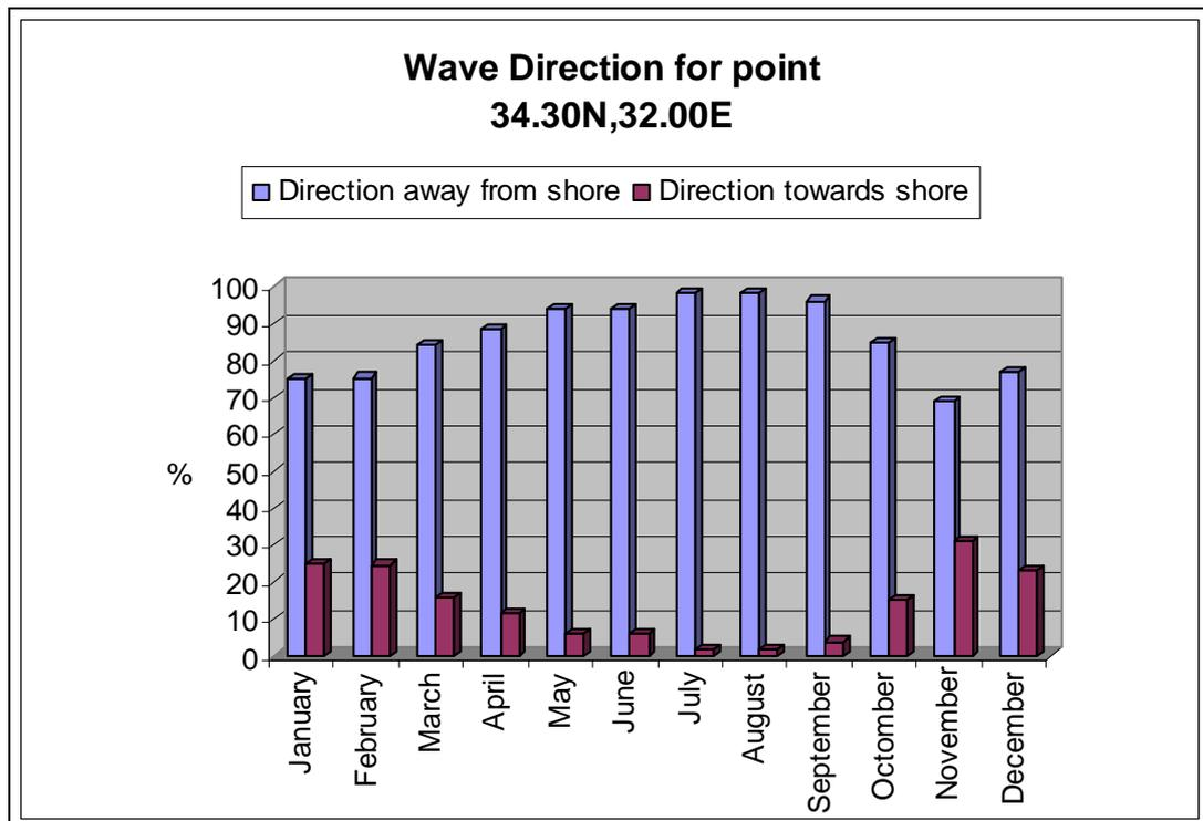
**FIG. 2: Distribution of Wave Direction for Point 34.30N, 32.00E (Vergetis et al., 2005).**
