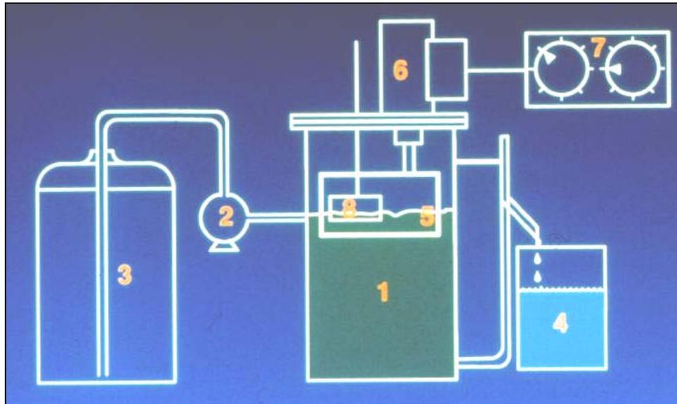
**Figure 2. Schematic drawing of IFP test apparatus. 1-dispersion vessel, 2-peristaltic pump, 3-seawater storage, 4-dispersed oil collection vessel, 5-oscillating hoop, 6-oscillating hoop motor, 7-motor controller, 8-oil containment ring.**
