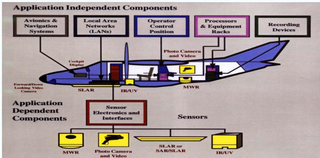
figure 1: aircraft lay-out
