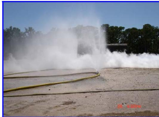
**Figure 3.** Water spray curtain and LNG vapors. Texas A&M Live Fire Training Workshop (2005).
