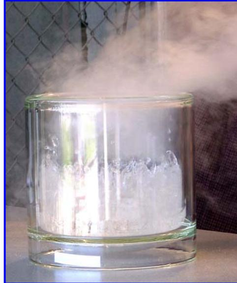
**Figure 2.** LNG vaporizing in an empty 1 gallon beaker – table top demonstration (Houston, 2002).
