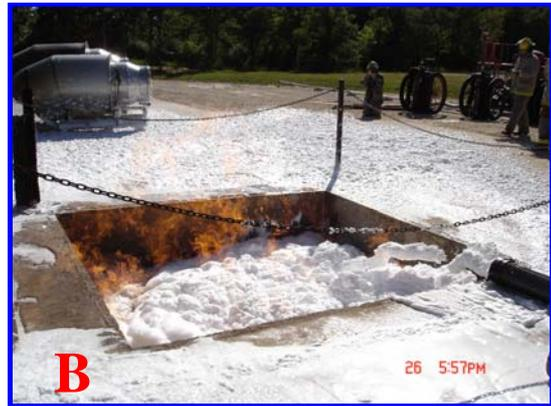
**Figure 5.** A. Medium expansion foam added to LNG fire in pit at Texas A&M Live Fire Fighting Workshop (2005).
