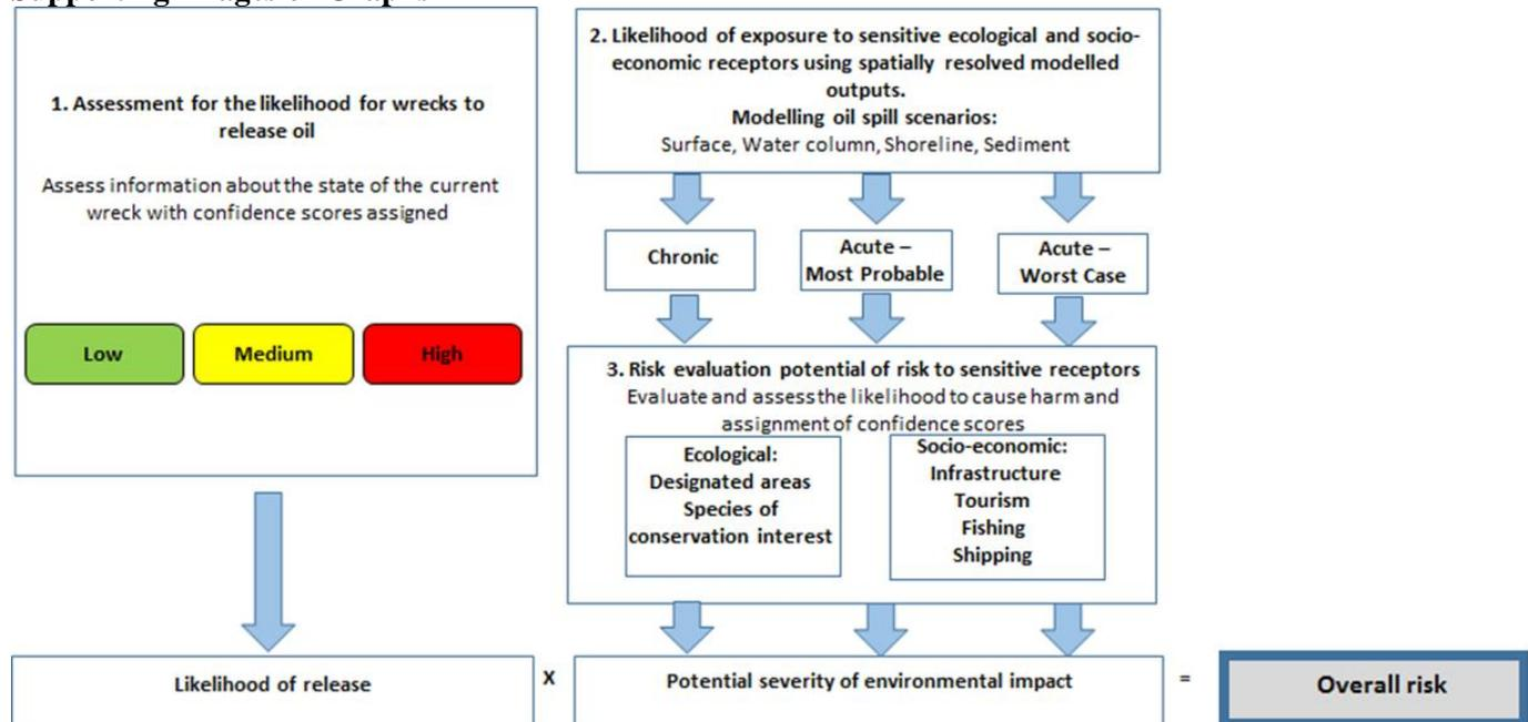
Figure 1: Flow diagram illustrating the E-DBA process).
