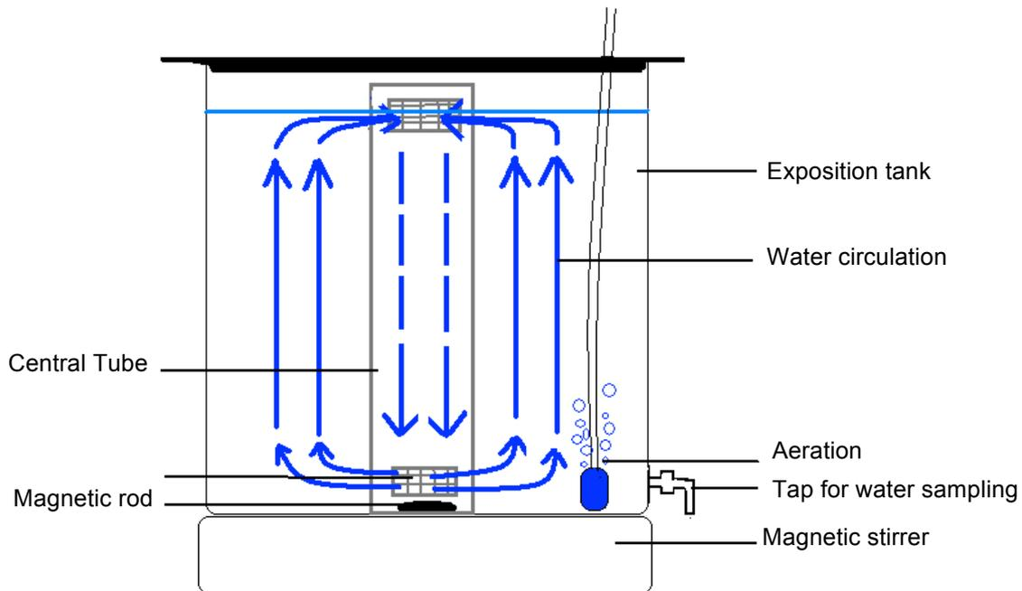
Figure 3: Exposure tank and water circulation
