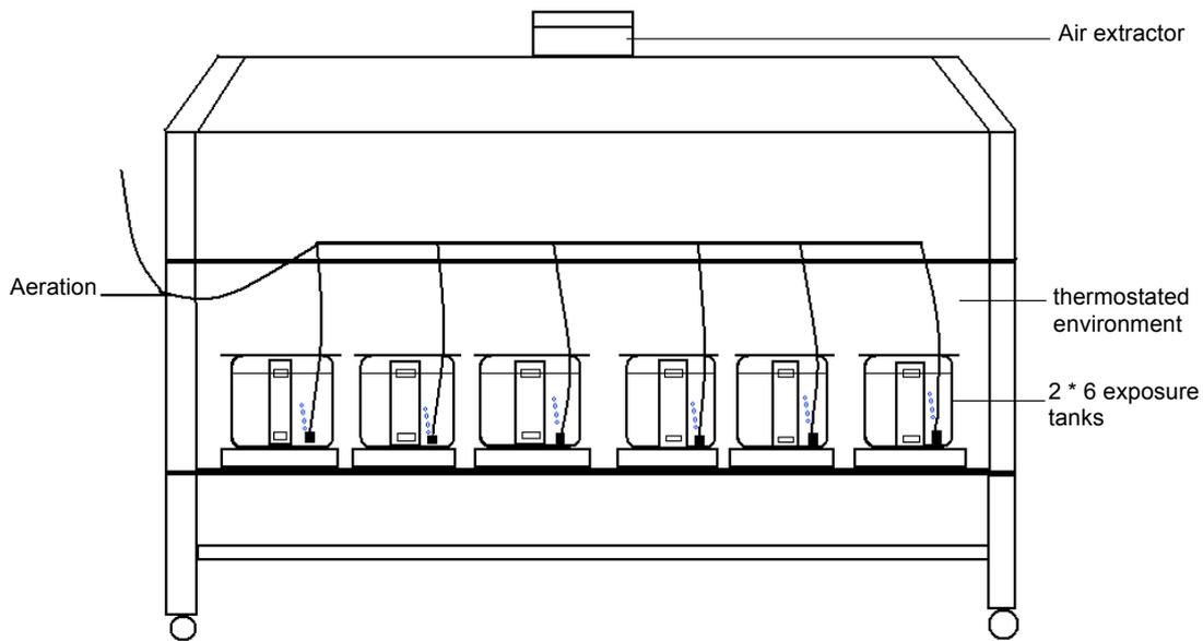
Figure 1: Side view of the ecotoxicological bench, showing the exposure tanks and the gaz inlet and outlet.
