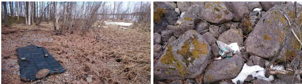
Figure 2. Target objects representing stranded oil (on left) and oil contaminated birds (on right). (Photos: J. Nevalainen)
