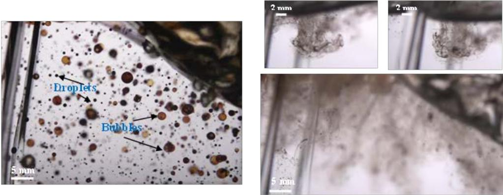
Figure 2: Oil behavior in turbulent flows: (left) oil alone without the addition of dispersants; (right) oil with dispersants, the DOR was 1:25. Experiments were conducted in baffled flask under rotational speed of 175 rpm.
