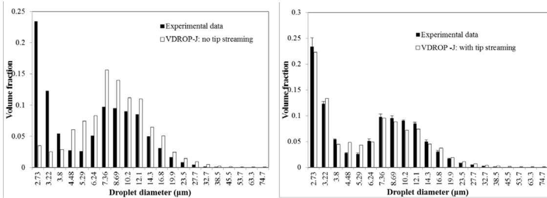
Figure 3: Comparison of the droplet size distribution predicted by VDROD-J (a) without and (b) with the tip streaming module with the experimental data.
