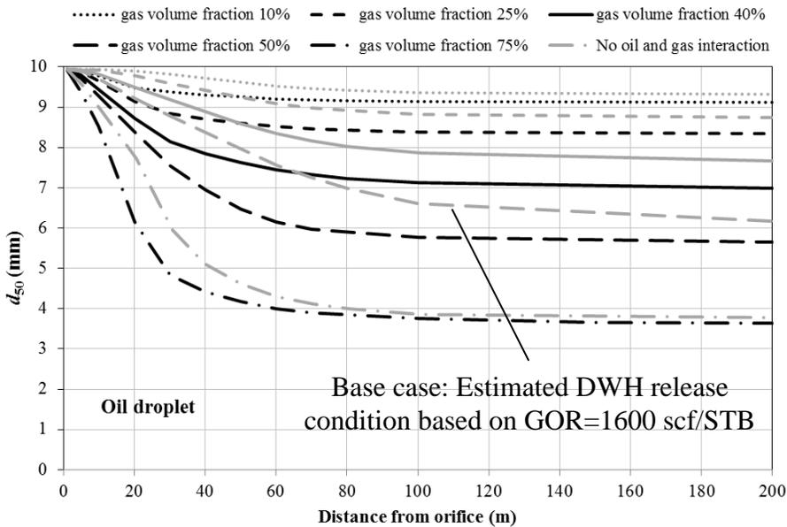
Figure 1: Evolution of the median droplet size  $d_{50}$  along the plume height for the cases without and with oil and gas interaction. The gas volume fraction 40% is the base-case with the GOR=1600 scf/STB.
