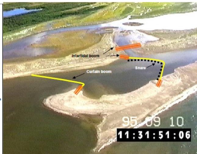
Figure 3 Example of flood tide control strategy at a small overlapping tidal inlet (narrow inlet with small tidal prism and sand beach shorelines)
