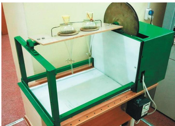
A laboratory test used to verify a dispersant product retains suitable effectiveness.
