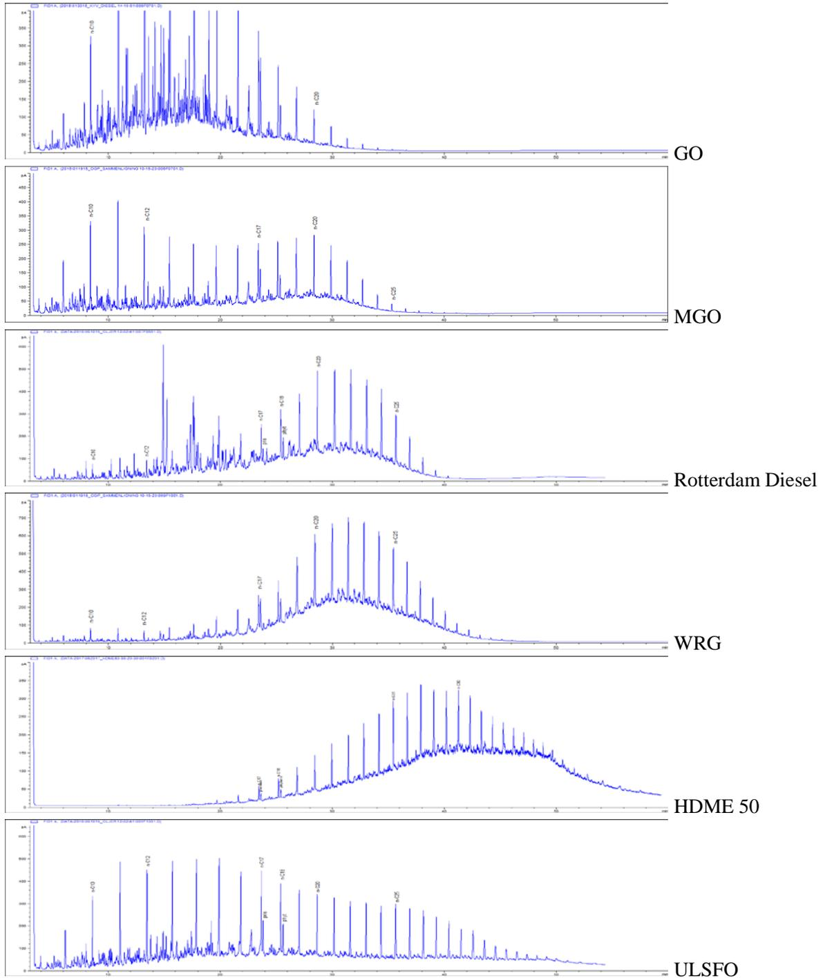
Figure 1: GC-FID chromatograms of the six tested fuel oils
