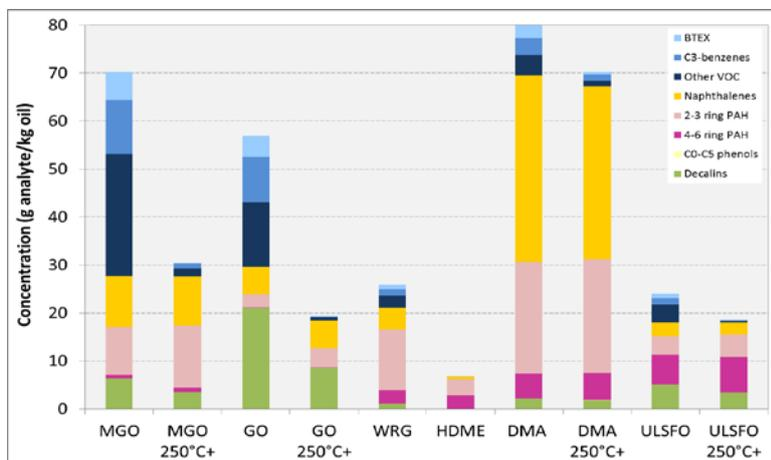
Figure 2: Chemical composition of selected component groups (aromatics) in the six fuel oils and their artificially weathered fractions
