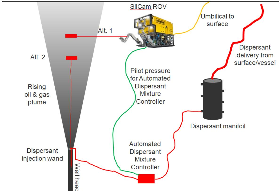
Figure 2: SSDI with automated dosage control and monitoring of effectiveness. Dispersant is injected into the well (Insertion tool), while the SilCam is used to monitor oil droplet sizes (SSDI effectiveness) and regulate dispersant dosage. The SilCam can either be positioned in the oil & gas plume by an ROV (alternative 1) or more permanently positioned in the plume (alternative 2).
