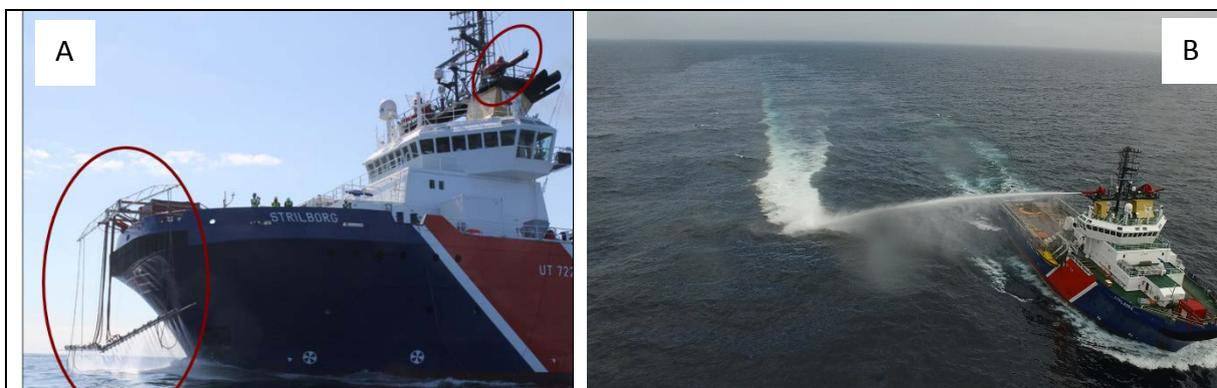
**Figure 2:** A: Response systems installed on MS Strilborg (low-dosage dispersant application followed by artificial turbulence using high-capacity water flushing bow booms)
