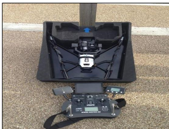
Figure 3 - UAS and Mobile Control Station (MCS) provided by Sky Futures – the MCS screen on the controls allows you to see what the UAS camera is filming
