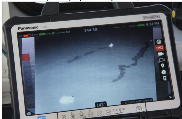
Figure 2 – shows the viewing screen, on the bridge of the Earl 2 vessel, illustrating the outputs of the Infra-Red sensor. The image shows two vessels and two lines of oil in the water (as the oil was released from the vessels).
