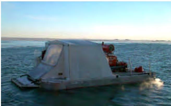
*Figure 10 The MORICE work platform during sea trials in Prudhoe Bay, Alaska, with a heated enclosure to avoid icing and freezing of equipment.*
