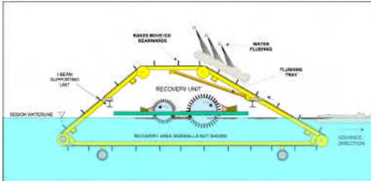
*Figure 9 MORICE ice processing and recovery principle: Larger ice pieces have oil flushed off while lifted out of the water by the grated belt, after which the ice is redeployed behind the unit. Oil and small ice goes through the grating where a recovery unit picks up the oil, possibly with some ice.*
