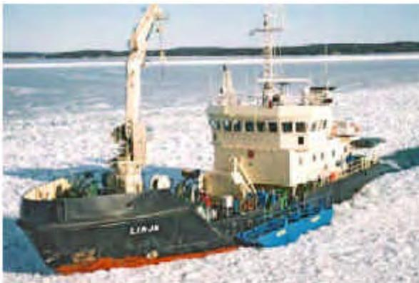
*Figure 8 The Vibrating Unit attached to the side of the vessel Linja.*
