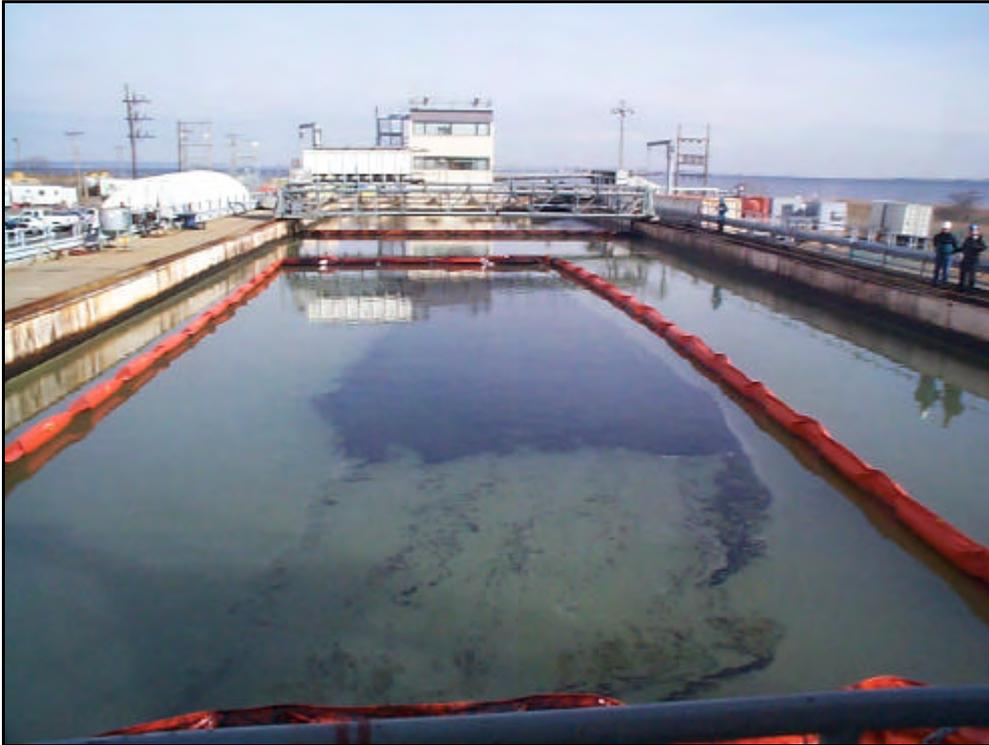
Figure 2. Ohmsett Test Tank with Oil Containment Boom
