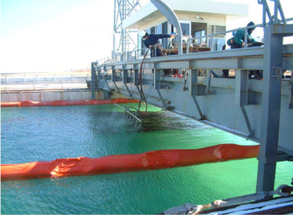
Figure 8. Dispersant Spray Bar in Operation During Testing
