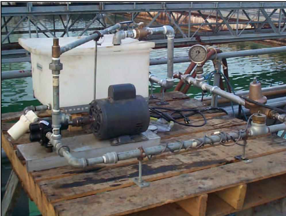
Figure 7. Dispersant Supply Tank and Pump
