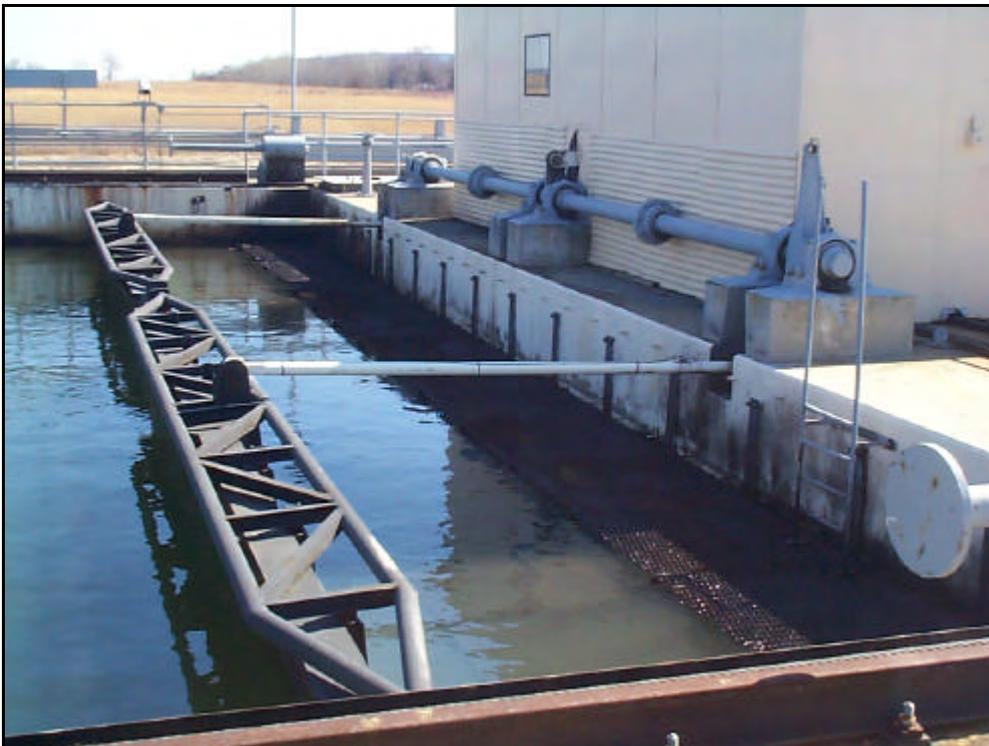
Figure 3. Ohmsett Wave Generator
