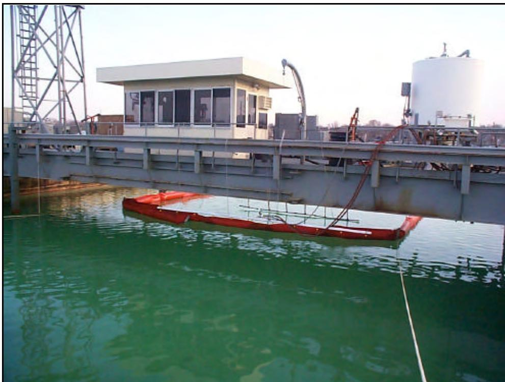
Figure 5. Main Bridge with Dispersant Spray Bar in Foreground, Oil Distribution Behind
