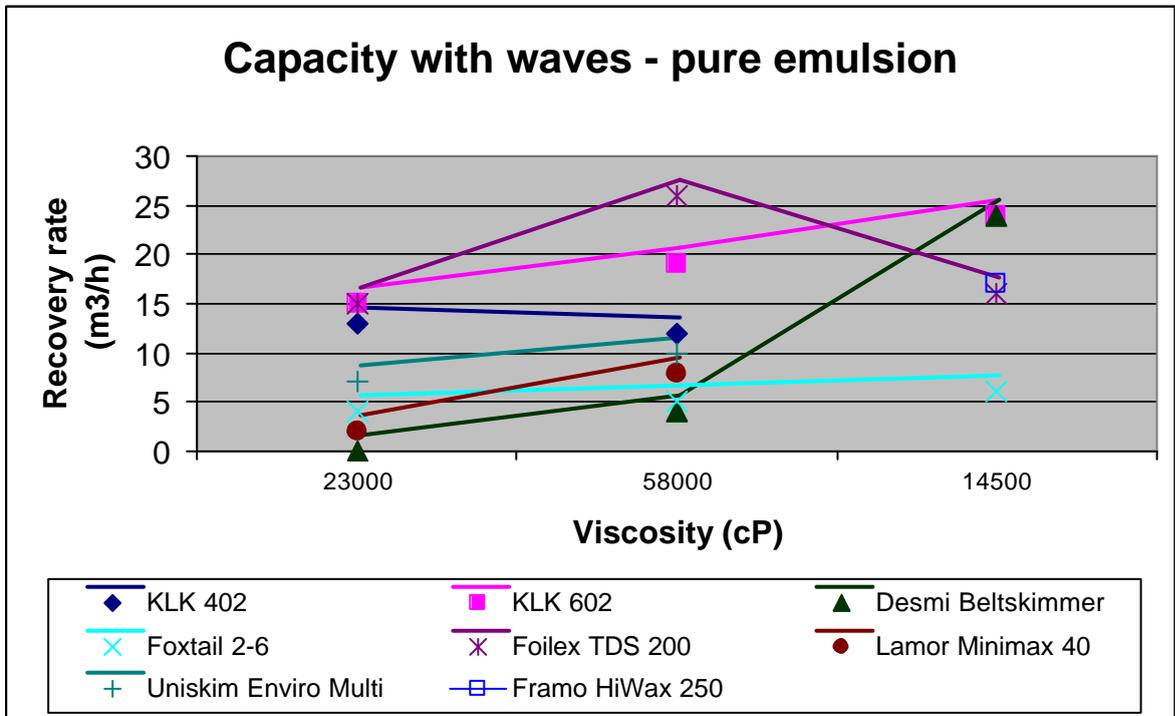
Figure 4. Recovery rate of pure emulsion vs. viscosity for all tested skimmers. 50 cm waves.
