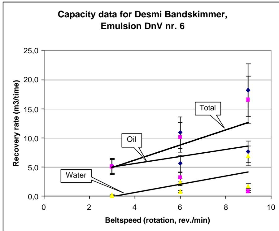
**Figure 2. Recovery rate of emulsion, free water and total fluid vs. belt speed for the Desmi Terminator belt skimmer in test emulsion no. 6. The size of the bars in the diagram represents 25% uncertainty in the measured recovery rate.**
