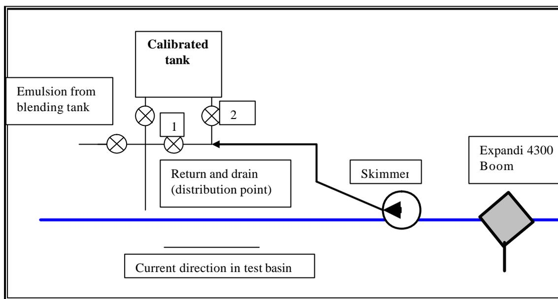
Figure 1. Illustration of the test set-up
