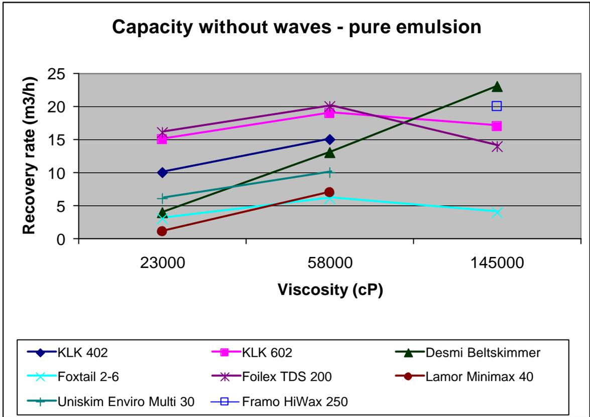
Figure 3. Recovery rate of pure emulsion vs. viscosity for all tested skimmers. No waves.
