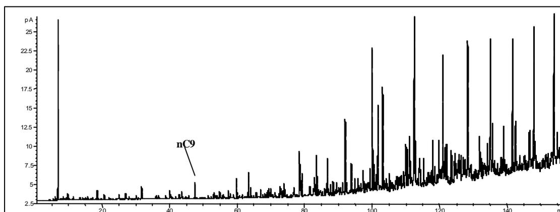
Figure 5: GC chromatogram of the C<sub>20</sub><sup>-</sup> fraction of the Prestige fuel oil n°6.
