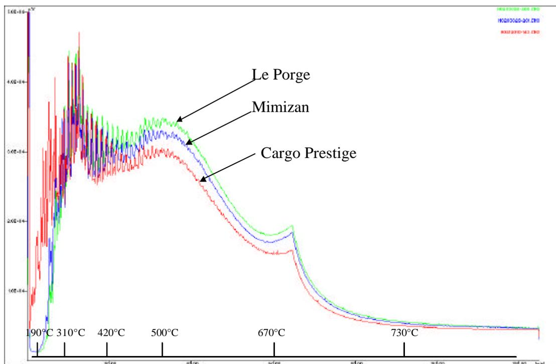
Figure 2 : High temperature chromatograms (simulated distillation) of heavy fuel oils originating from the Prestige cargo and different beaches.
