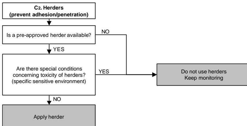
**Figure 8** Decision tree to determine if herders can be used to prevent adhesion/penetration
