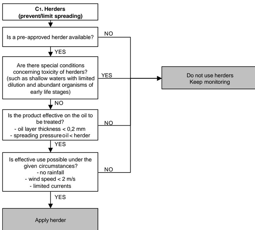
**Figure 7** Decision tree to determine if herders can be used to prevent/limit spreading
