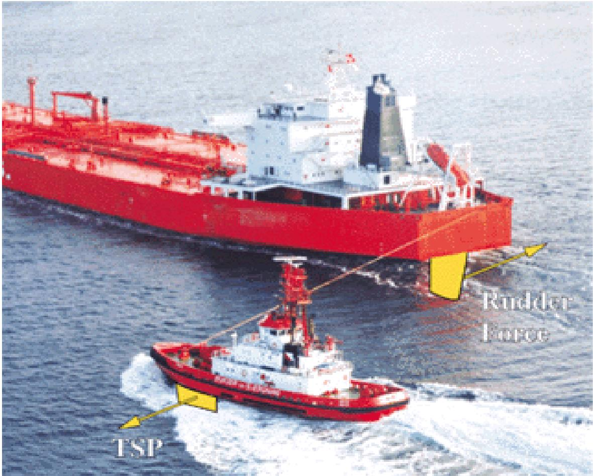
Tug escorting of ships requires Tonnes of Steering Pull - **TSP** - at higher speeds for emergency steering. Every year our tugs escort thousands crude oil and gas-carriers at terminals in Norway, which may prove useful also for salvaging and towing tankers in distress.
