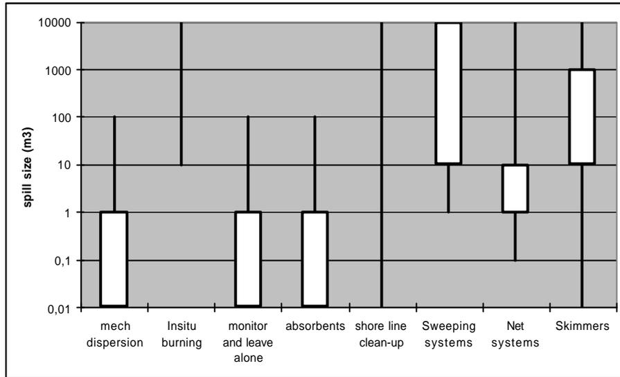
**Figure 1 Feasibility of a few response options as a function of the spill size**
