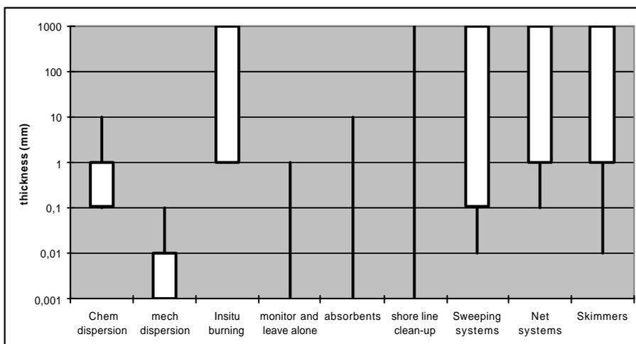
**Figure 2 Feasibility of a few response options as a function of the spill layer thickness**
