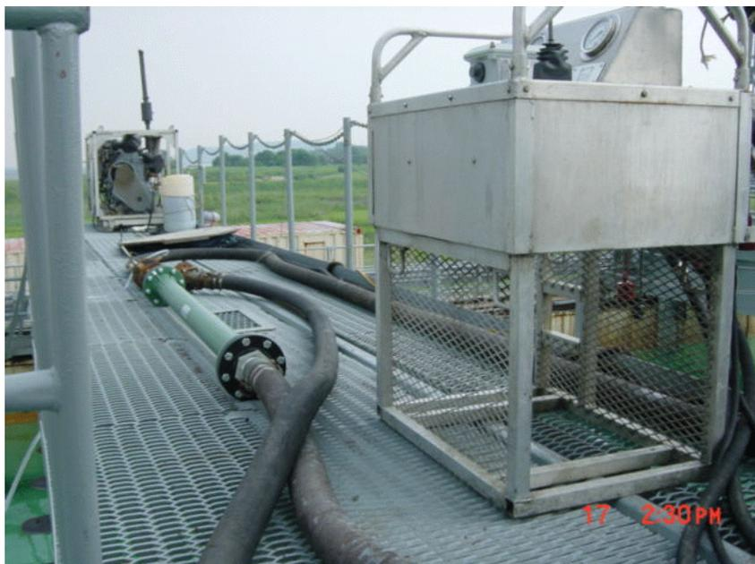
Figure 9. In-line mixer on deck connected to discharge hose just before recovery tanks.
