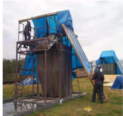
**Figure 6. Shading and Water Cooling of the Canadian Coast Guard Test Tank.** A sprinkler system enhanced evaporative cooling. Two temperature probes were monitored daily. Tank was insulated just before testing.
