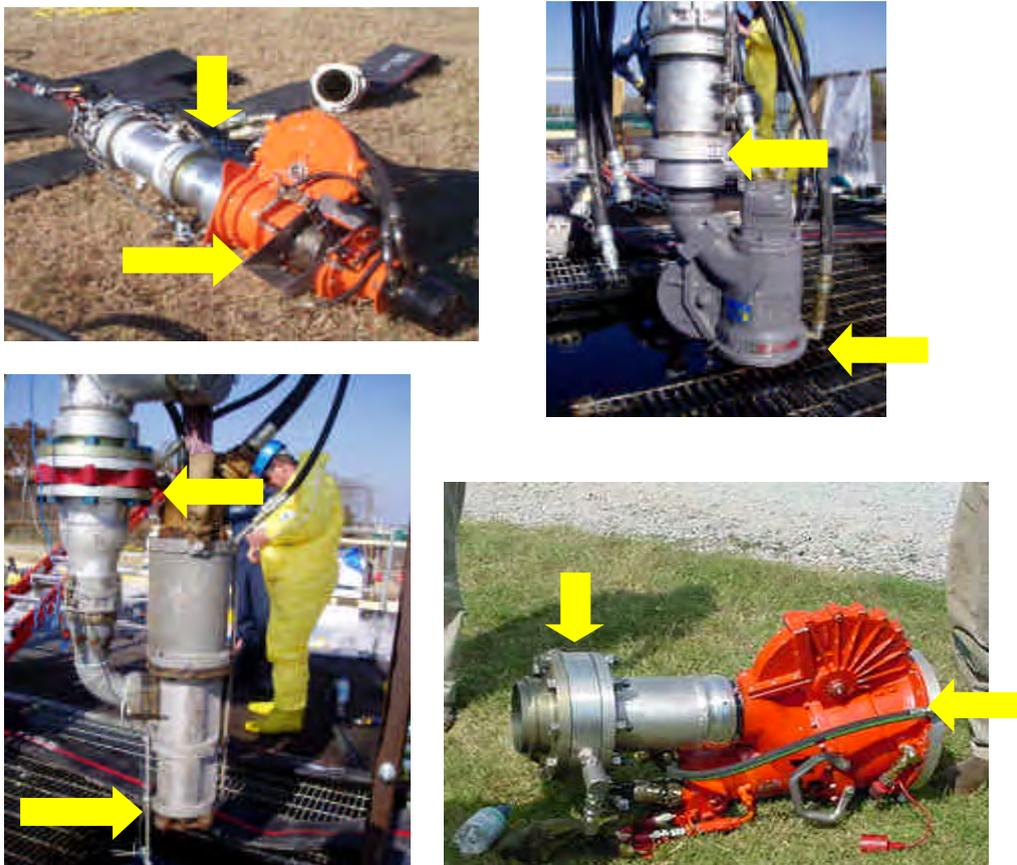
**Figure 1. The Pumps Tested at the JVOPS Workshop. Clockwise from left-top: Canadian Coast Guard GT185, Lamor GT-A 50, U.S. Coast Guard Desmi DOP-250, and Framo TK-125. The arrows denote the inlet and outlet water lubrication devices within or attached to each pump.**
