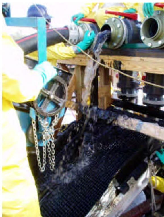
**Figure 25. The SHAS and ERE Belt Skimmer. The Environmental Recovery Equipment (ERE) Skimmer sat atop the CCG Test Tank and separated lubrication water from the returning Test Product for follow on tests.**
