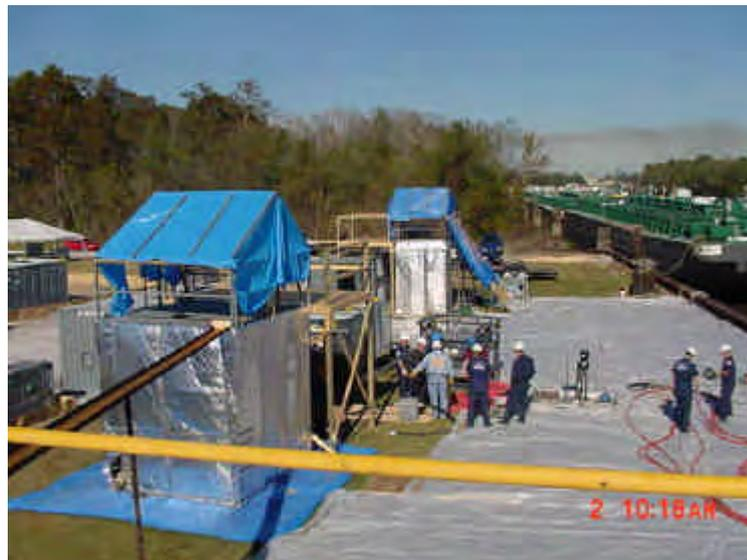
**Figure 7. The USCG Test Tank (foreground) and Canadian CG Test Tank (background) From Atop the Baker Tank.** Once the Test Product assimilated to the average ambient temperatures and resulting target viscosities were achieved, insulation was added to the tanks in November to maintain viscosities.
