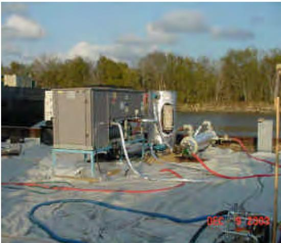
**Figure 10. The Chiller System. This was essential to maintain target viscosities for both USCG and CCG Test Products. The system was closed-loop ensuring no oil contamination of the bayou or ground.**
