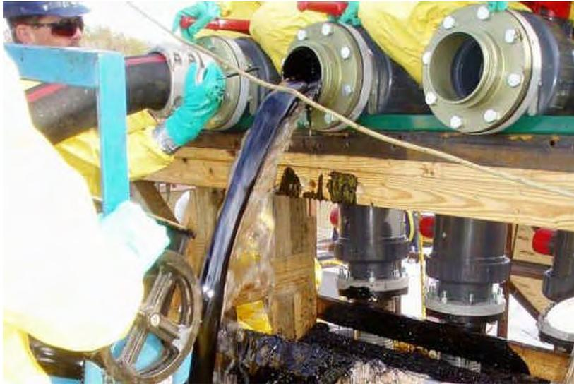
Figure 27 Discharge of 480,000 cSt oil and lube water in 150 m test with GT-185
