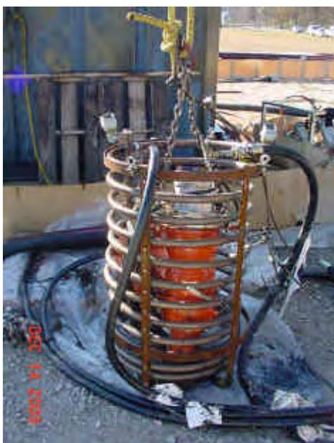
**Figure 26 (left). U.S. Navy Steam Coil Around GT-185 Pump.**
