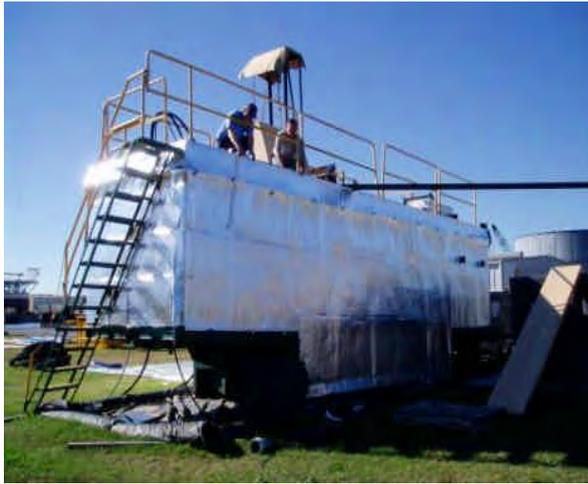
**Figure 5. The Baker (Backup) Tank.** It was shaded prior to testing, then insulated just prior to and during testing. Test Product was re-circulated within for 2 months prior to actual testing. A water sprinkler system was installed (under insulation) to enhance evaporative cooling. Nine temperature probes within were monitored on a daily basis before and during testing. .
