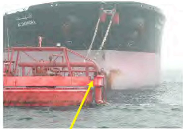
Figure 4 – Offshore Loading Buoy with Sensor & Alarm
