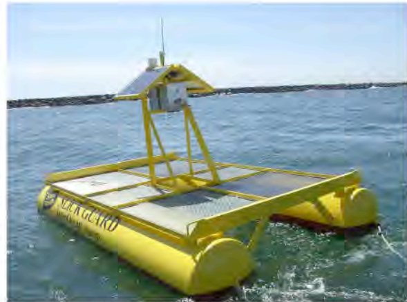
Figure 5 – "Slick guard" Buoyancy Platform Environmental Sensor System
