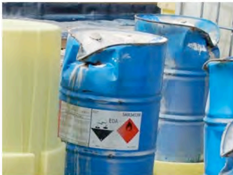
Fig. 6 Pressure damaged drums of EDA
