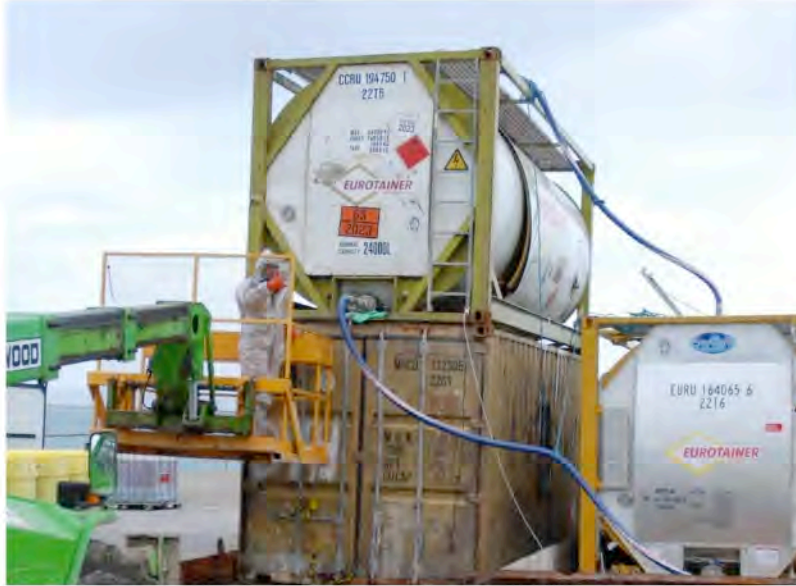
Fig. 5. Tank container of Epichlorohydrin being transferred under gravity
