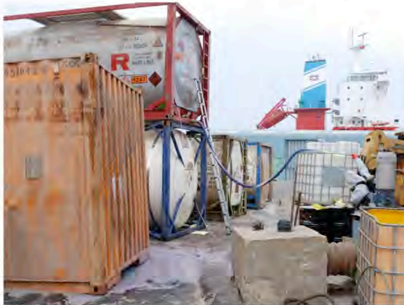
Fig. 9 Preparing to Add Inhibitor to a Tank Container of Methyl Methacrylate by Bleeding off some of the contents to an IBC.
