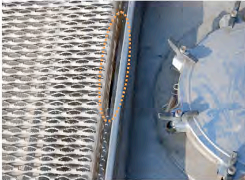
Fig. 8. Damage to Tank Container of Methyl Methacrylate
