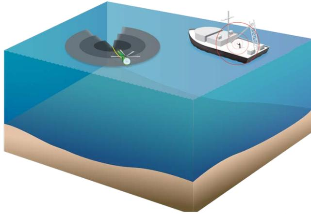
Figure 1. Detection of slick thickness using a towed platform
