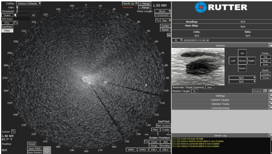
**Screenshot of Radar detecting Oil and Infrared Camera view used to visually identify**
