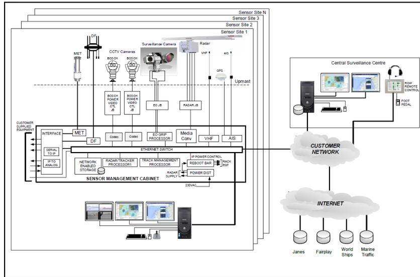
**Typical Network Architecture (Drawing Courtesy of Raytheon Anschutz)**
