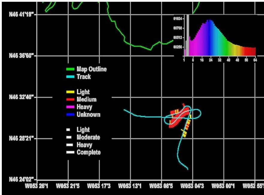
Figure 1 Portions of a real-time fluorosensor output display. The oil detections are shown as bars along the mapped flight path. The color of the bars shows the type of oil measured. The length of the bar shows the aerial coverage. At each point along the flight path the spectrum of the target is also displayed (From Environment Canada)
