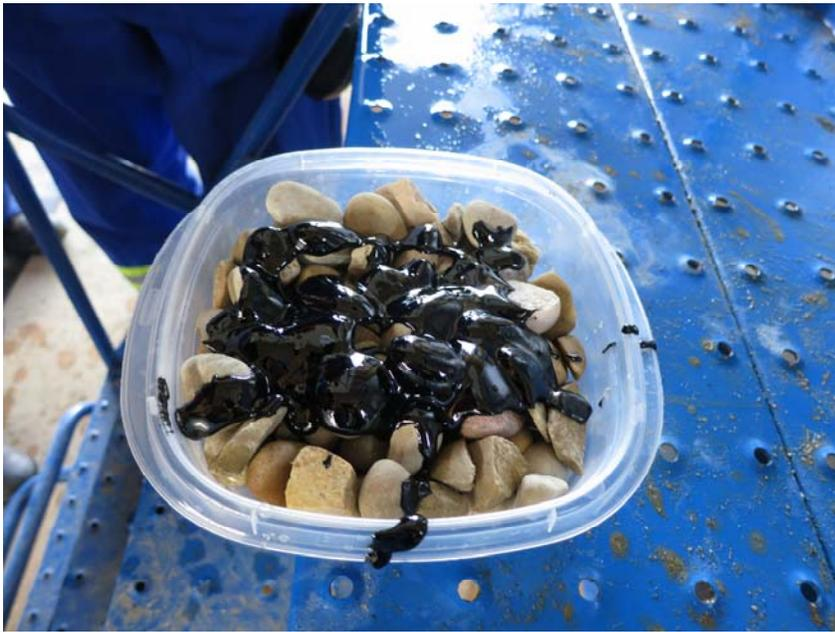
Figure 15 Test of weathered Dilbit gravel penetration – Gainford Tests – May 2013
