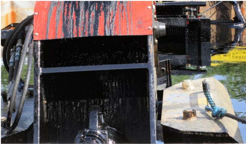
Figure 17 A Lamor skimmer operating during a weathered Dilbit recovery test
