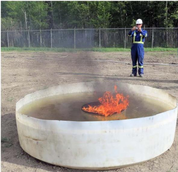
Figure 19 A test burn of weathered Dilbit
