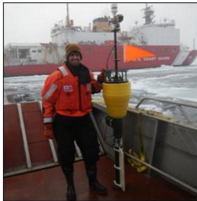
**Figure 5. Surface Wave Instrument Float with Tracking (SWIFT) Buoy.**
