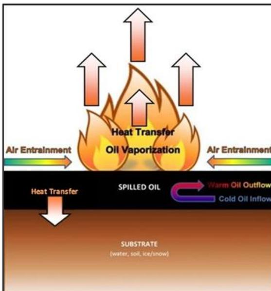
**Figure 2. Schematic of the movement of air and transfer of heat from an in-situ burn** (modified from Fritt-Rasmussen, 2010).
