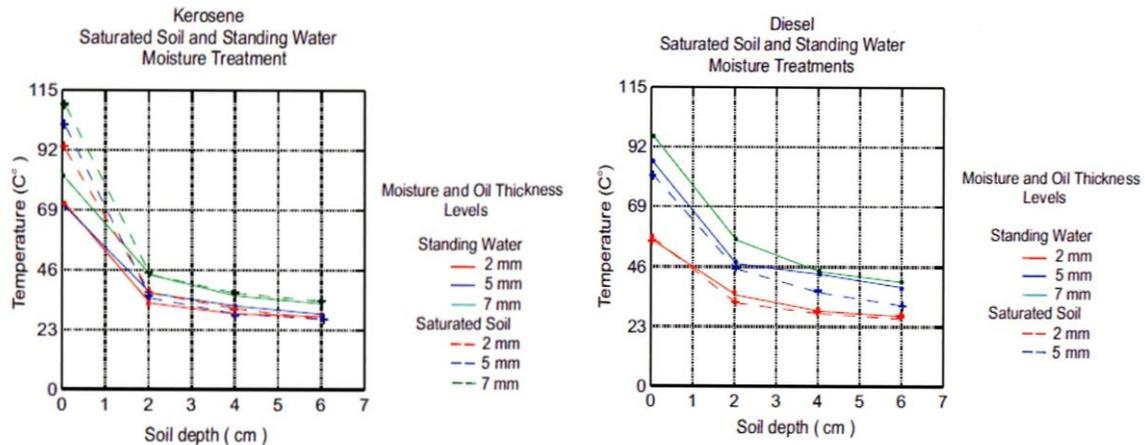
**Figure 7. Kerosene and Diesel Maximum Soil Temperatures in Saturated Soils.**
