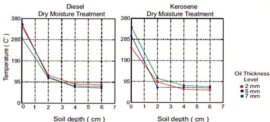
Figure 5. Diesel and Kerosene Burn Maximum Soil Temperatures of the Dry Soils.
