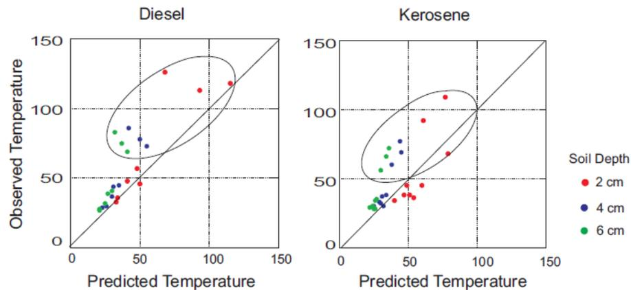
**Figure 8. Comparison of diesel and kerosene burns' observed and predicted temperatures. The dry soil treatment temperatures are within the ellipsoids.**
