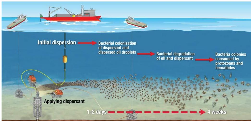
**Figure 2.** Diagram illustrating SSDI and the subsequent biodegradation process that begins when dispersants are applied to a deepwater release.
