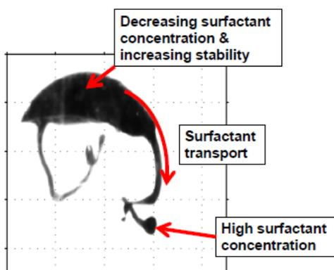
**Figure 10.** Drawing illustrating the movement of surfactants in an oil droplet during “tip streaming.”
