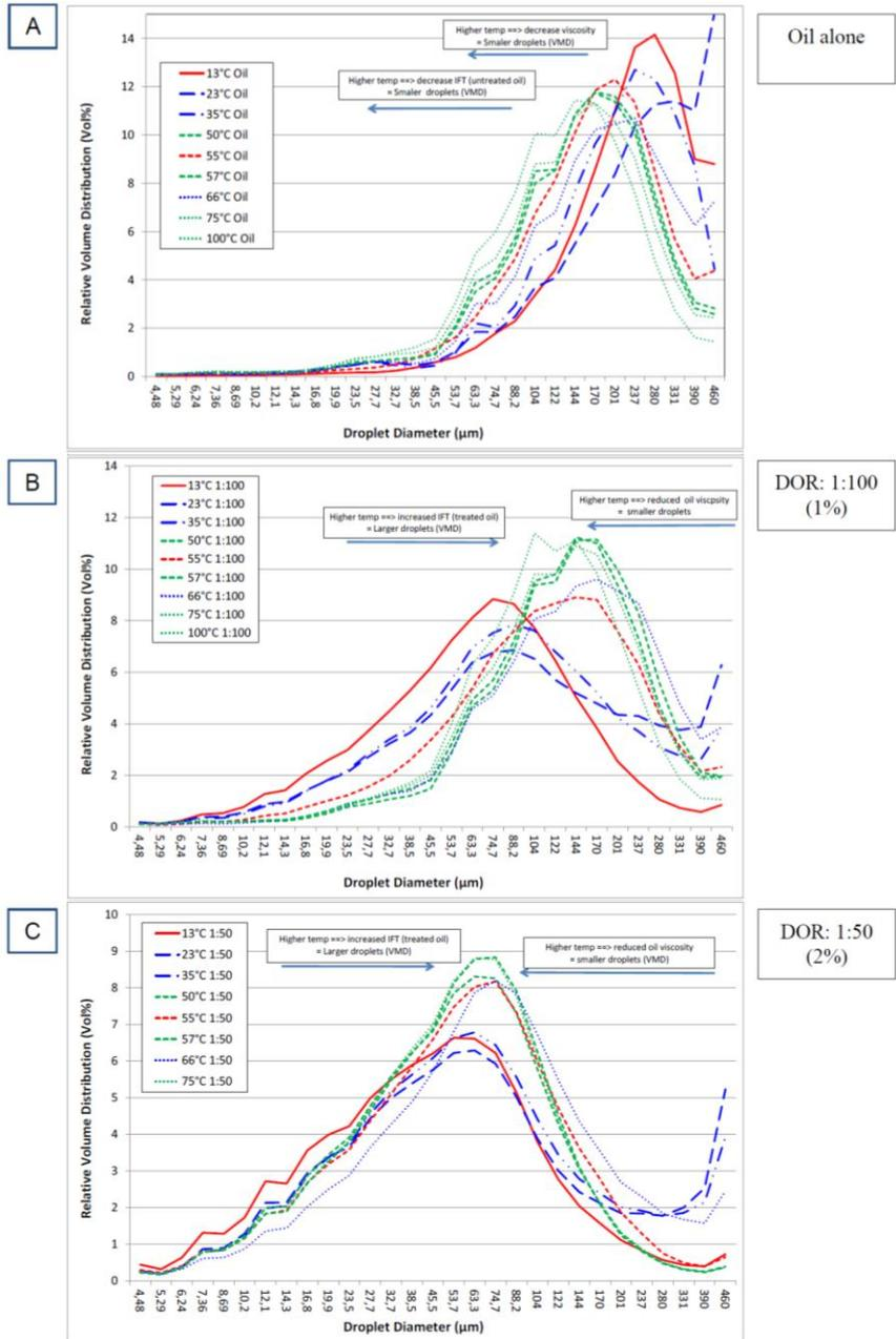
Figure 12. Combined results from the three different tower tank experiments as a function of temperature (13-100°C). A: oil alone, B: DOR: 1:100 and C: DOR: 1:50.
