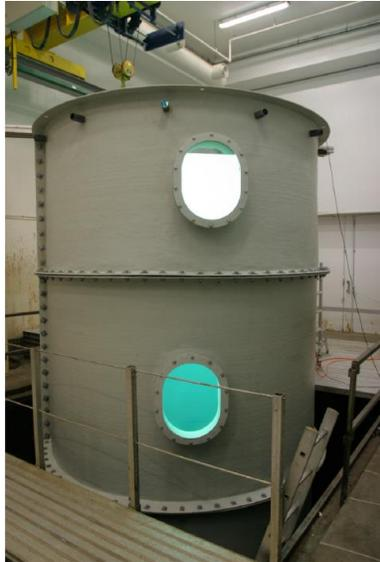
**Figure 4.** Photo of the 6 m tall by 3 m diameter tower tank used to conduct scaled experiments of SSDI.
