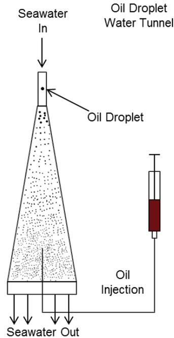
**Figure 8.** Conceptual drawing of the inverted-cone water tunnel used to study the far-field behavior of droplets.
