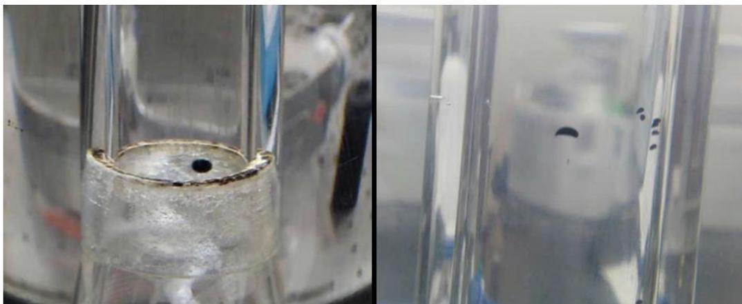
**Figure 9.** Images of droplets suspended in the inverted-cone water tunnel. The image on the left shows a typical ball-shaped untreated oil droplet and the image on the right shows the inverted-bowl shape seen when a droplet was treated with dispersant (DOR was 1:50).
