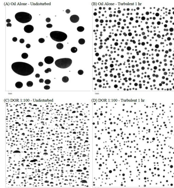
**Figure 11.** Digitized images of droplets in the inverted-cone water tunnel showing (A) untreated droplets immediately after they are injected into the tunnel, (B) untreated droplets after experiencing 60 minutes of continuous water down flow in the tunnel, (C) treated droplets (1:100 DOR) immediately after injection into the water tunnel, and (D) treated droplets after 60 minutes of continuous water down flow in the tunnel.
