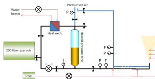
**Figure 5.** Drawing showing the set-up for the tower tank to allow study of SSDI.
