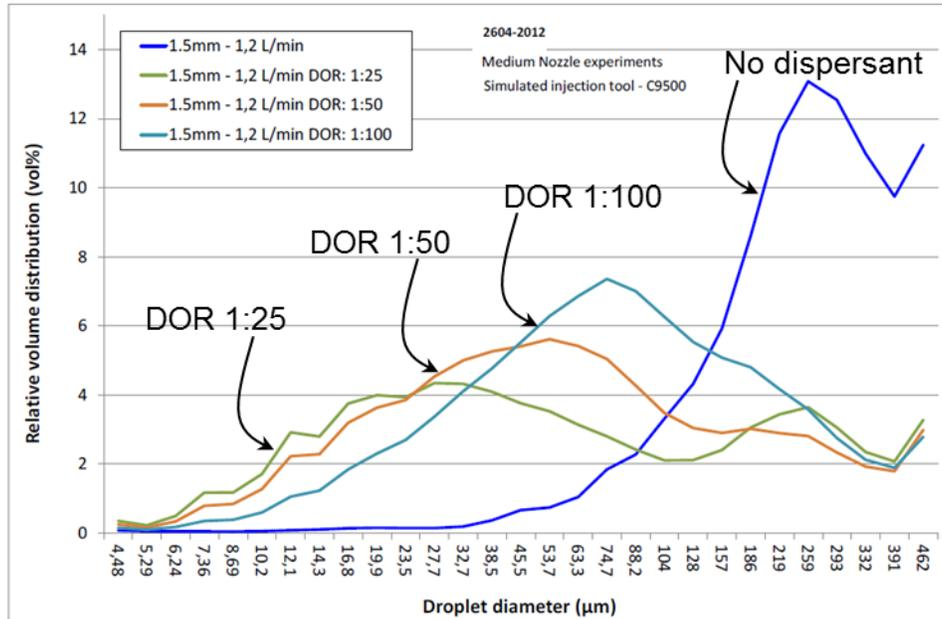
**Figure 6.** Droplet size distribution (volume %) formed for different DORs. Release conditions were a 1.5 mm diameter discharge port and an oil flow rate of 1.2 L/min.
