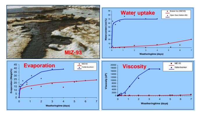
*Figure 1* Comparison of weathering parameters from the Barents Sea Marginal Ice Zone (MIZ) experiment in 1993 with similar data from open water field experiments.
