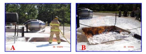
Figure 5. A. Medium expansion foam added to LNG fire in pit at Texas A&M Live Fire Fighting Workshop (2005).B. Foam blanket on LNG fire in pit (2005).
