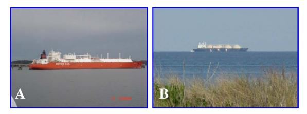
Figure 1. A. LNG vessel at berth (membrane-type cargo tanks);B. LNG vessel underway (Moss-spherical cargo tanks).
