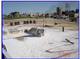
Figure 6. Turbex high expansion foam generator at Texas A&M (manufactured by Angus Fire Company).
