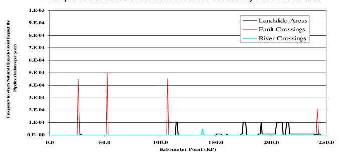
Figure 3 Example of Out from Assessment of Failure Probability from Geohazards
