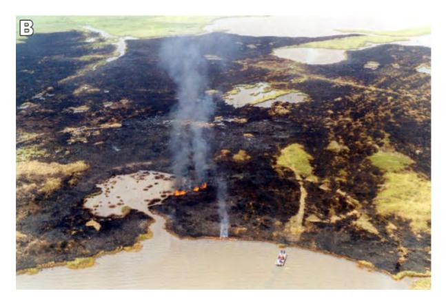
**Figure 6** – This picture of Mosquito Bay was taken one hour after the first burn ended. The arc around the small bay is the attempted firebreak. The straight line across the upper right traces the pipeline. The spill source is off the page to the right (API, 2002).
