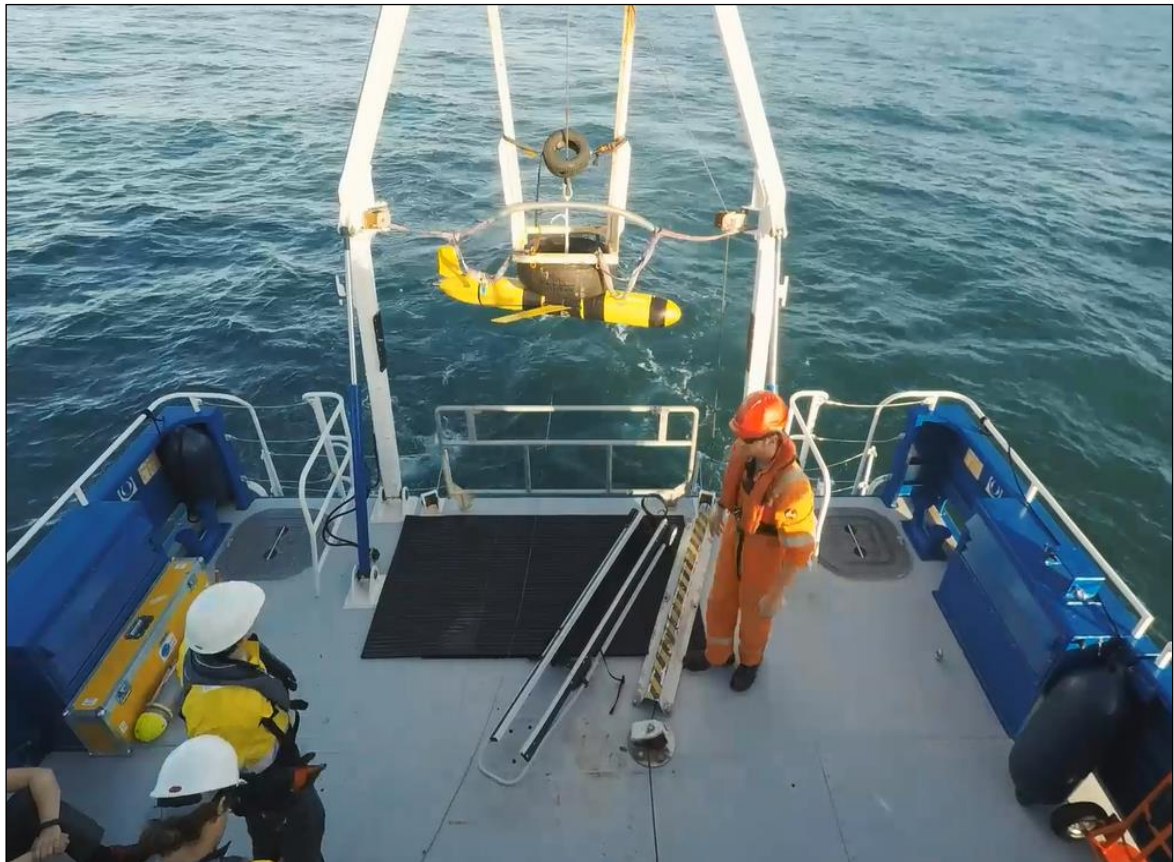
Figure 5 – The Slocum Glider AUV launching from the Solent Guardian
