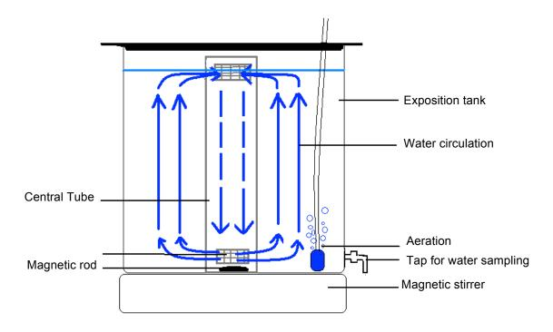
Figure 3: Exposure tank and water circulation
