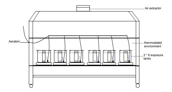
Figure 1: Side view of the ecotoxicological bench, showing the exposure tanks and the gaz inlet and outlet.
