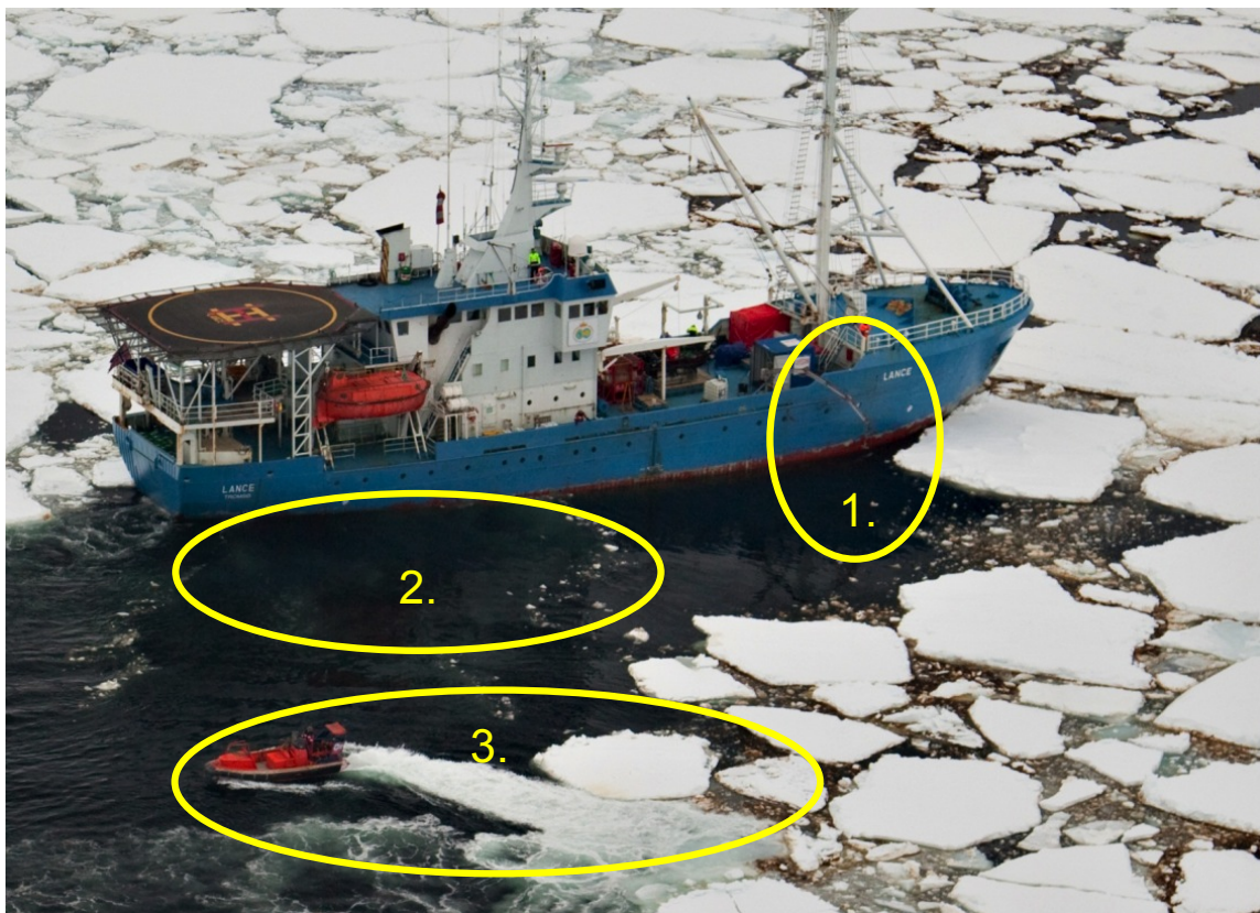
Figure 3: Overview of the dispersant application strategy used during the field trial in the Barents Sea
