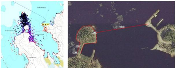
Figure 1. Incident scenario illustrating the oil drift modeling and shoreline contamination. The colours represent the extent of the spreading in given time intervals. On right hand side, the location of the Incident Command Post. (Graphic: J.Kauppinen, maps: ©Liikennevirasto, ©Maanmittauslaitos, ©Boris)
