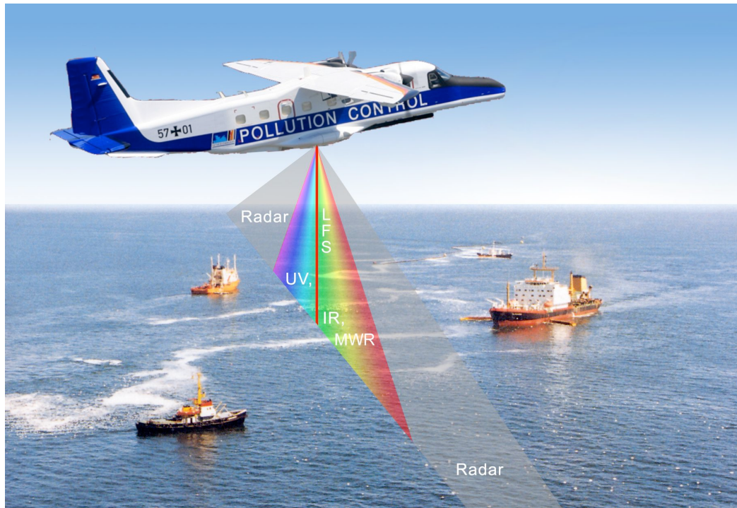
Figure 3: Schematic demonstration of the different line sensors on board of an aerial surveillance aircraft (example from Germany)
