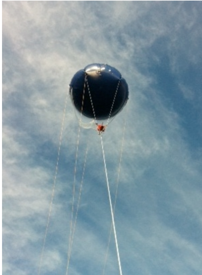
Figure 8. Aerial Observation Spill Response Balloon
