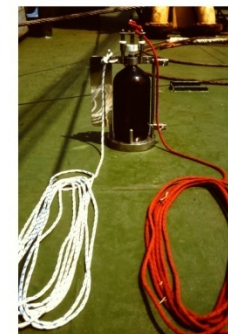
Figure 6. Cefas shallow water sampler rigged for use. The sampler is lowered using the white rope, and opened and closed using the red rope.
