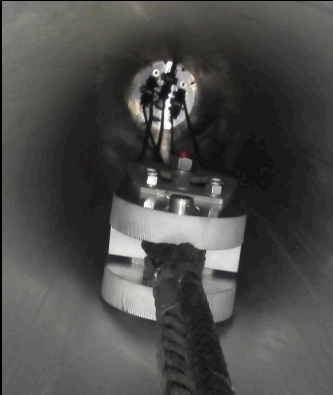
'anti-tilt' rig inside mast
