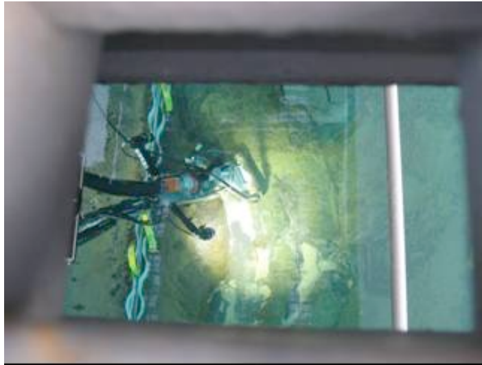
Figure 4. Heated nozzles removing oil from tray (bottom of tray exposed)
