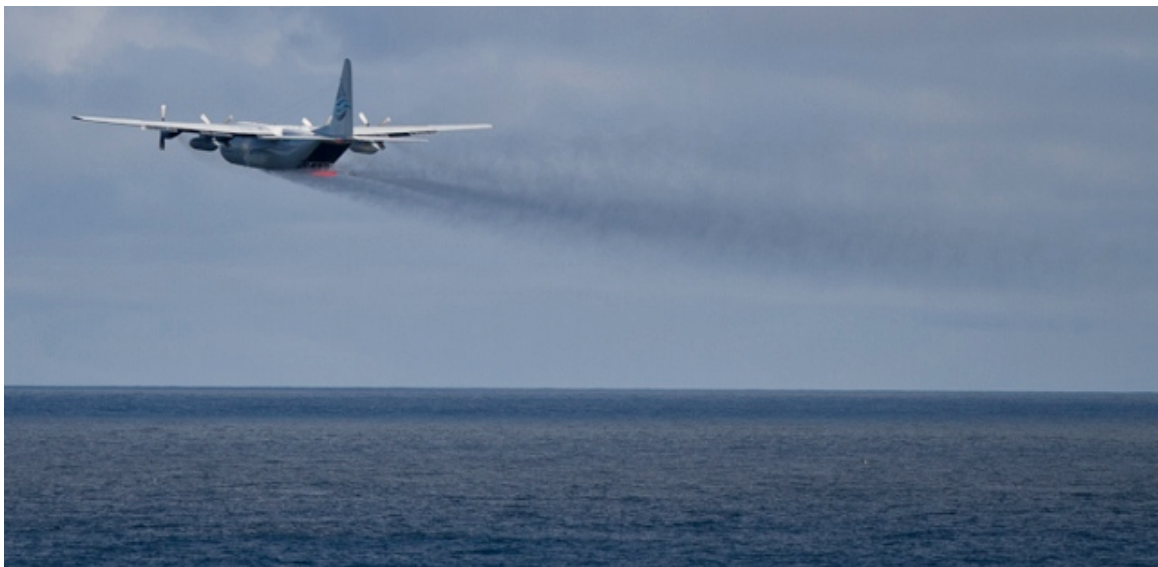
Figure 2. OSRL Hercules dispersant application. Guidance was provided by the Norwegian surveillance Beech 200 aircraft LN-TRG.
