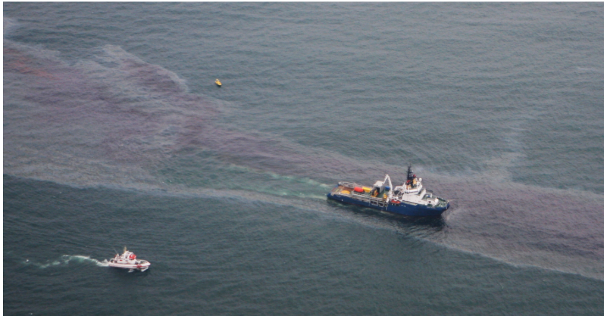
Figure 4. M/V Stril Power during dispersants application.
