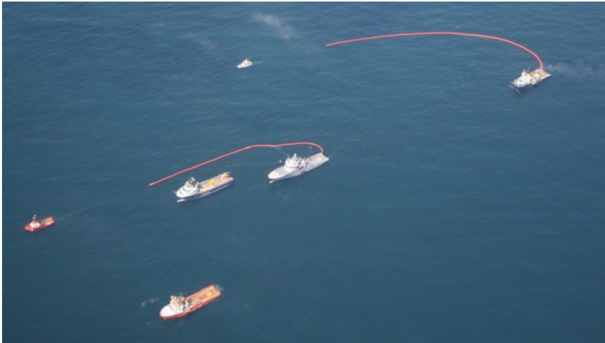
Figure 3. M/V Stril Mermaid releasing emulsion into the boom of Coastguard vessel Bergen. Backup system of M/V Stril Power seen aft.
