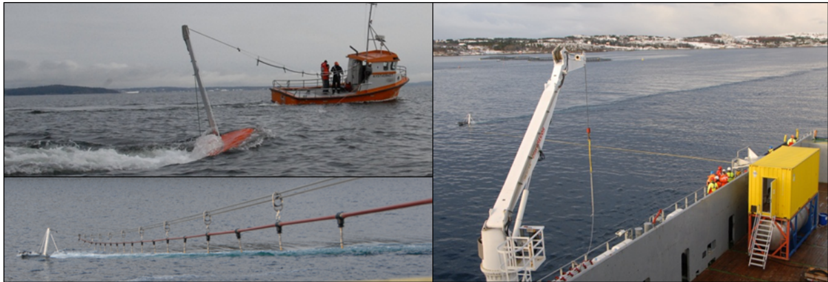
Figure 5. Dispersant application system using paravane, coastal version with 20 m swath width (upper left) and offshore version with 50 m swath width.
