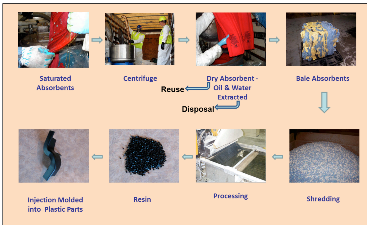
Process flow diagram of soft boom recycling into plastic parts
