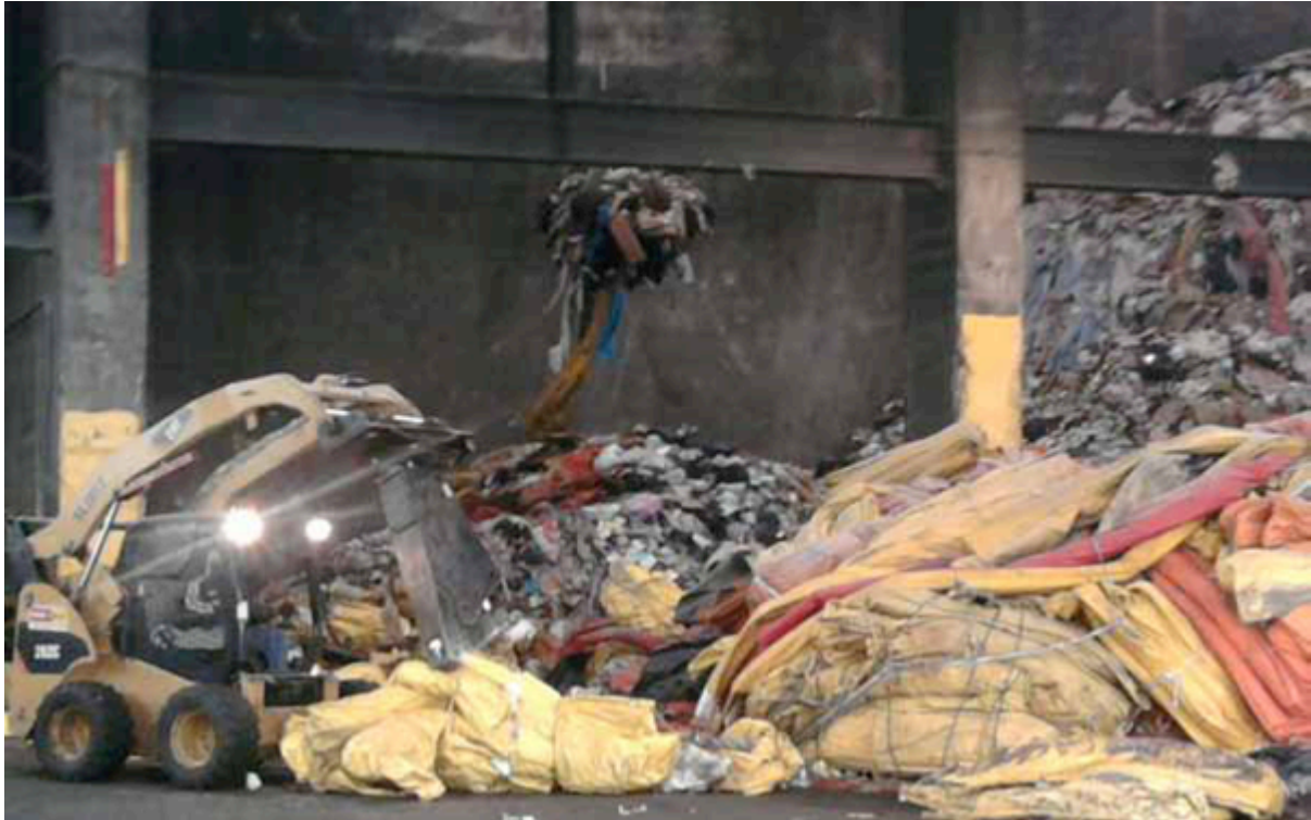
Figure 3- Hard boom being processed on the tipping floor at a WTE facility
